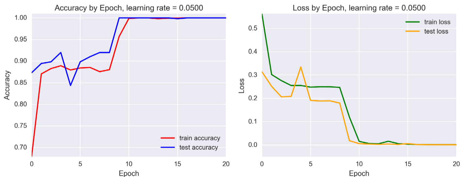
Figure 18.53: Accuracy and loss for our network when using a learning rate of 0.05.
