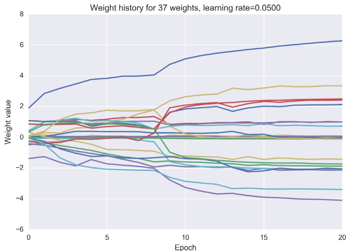
Figure 18.54: The weights in our network over time, using a learning rate of 0.05.
