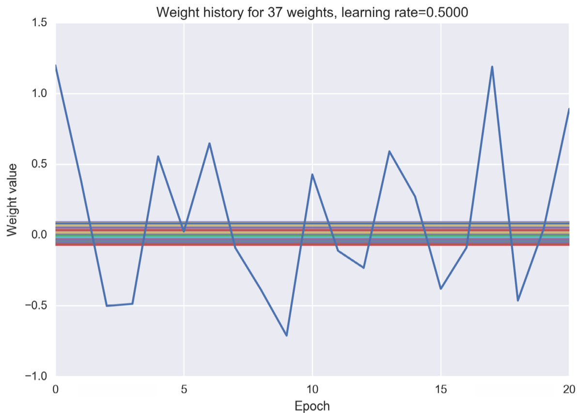
Figure 18.51: The weights of our network when using a learning rate of 0.5. One weight is constantly changing and overshooting its goal, while the others aren't making any visible changes.
